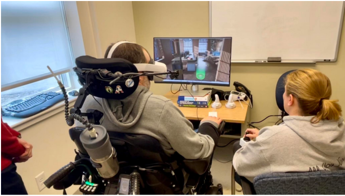
Fig. 1. Photo of our preliminary study. A participant who uses a chin-controlled wheelchair is interacting with the VR training system and orally giving instructions to control the virtual wheelchair via our standard joystick.
